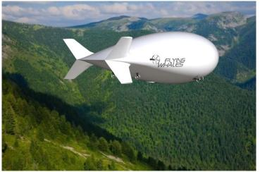
FLYING WHALES' LCA60T is a "rigid" airship; it has a cargo hold or under-sling payload capacity of 60 metric tons and a cruising speed of about 100 km/h. It benefits from the same operational flexibility as a helicopter (point-to-point, overcoming the constraints of transport infrastructure or geographical obstacle, and loading/unloading its freight while hovering), but its operating cost per transported ton will be twenty to forty times lower than the latter.
