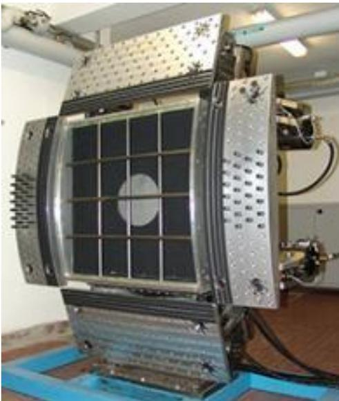
Figure 3: Example of fuselage panel test (courtesy AESDO/POLITO)
