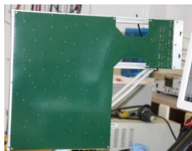
Figure 2: Example of microphone array containing 64 sensors.
