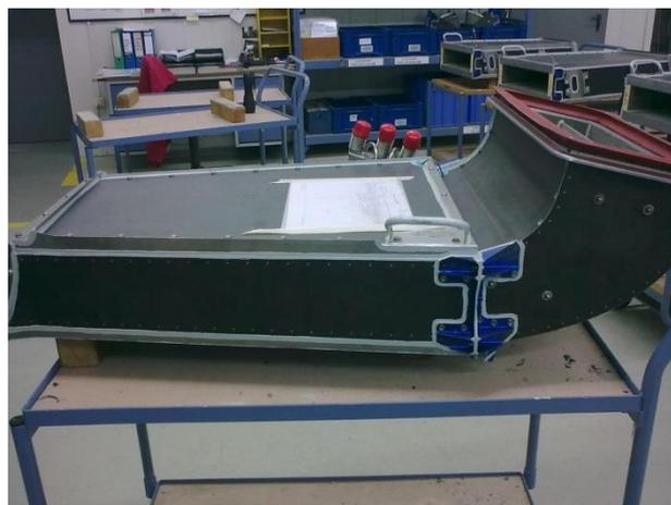
Figure 4 Example of Air intake ducting
