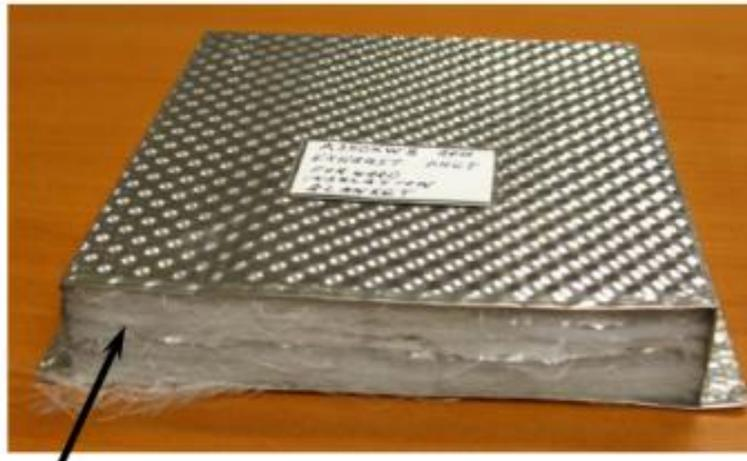
Figure 2 – Typical thermal blanket for exhaust mufflers
