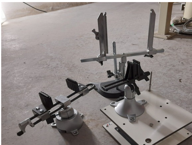
Figure 3: Selection of PANAVISE instruments for DUT positioning
