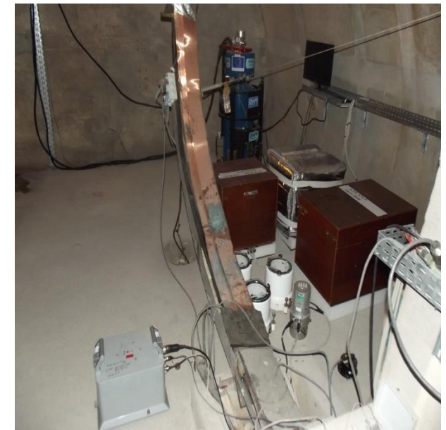
Comparison of gravimetric, micro-barometric, velocimetric, accelerometric measurements in a broad frequency band
